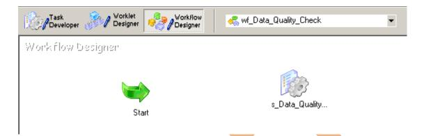
**Step-5** Now create flow B/W Workflow to Task. Select Line Task and link to Start to s\_Data\_Quality\_Check.
