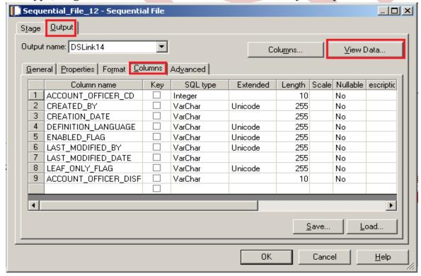
Step-16:- Now click on View Data and Ok. If your data is shown like this that means you have made successful connection between input file and Datastage otherwise it will give some error like column mismatch error.
