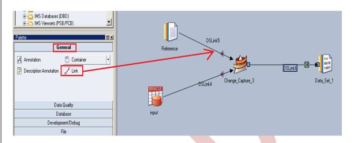
**Step-7:-** Now double click on oracle stage to fetch oracle table into DataStage. There are multiple methods available, We choose table as Read Method as we know the table and schema name so we directly call the table.
