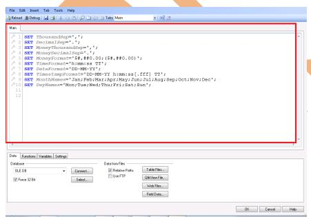
**Step 6** Now the data records as in the form of access,qvd or excel sheet this covers the procedure extract which is the fundamental procedure of datawarehousing by connect option we import the access file in which records are saved. Select the Database connection type from Data tab in the Edit Script window as shown below:
