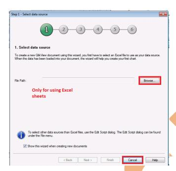
If you want to use data source different from Excel format like access or qvd data source going through this process->Click on "Cancel", so that we can save the document with the blank datamodel and dashboard.
